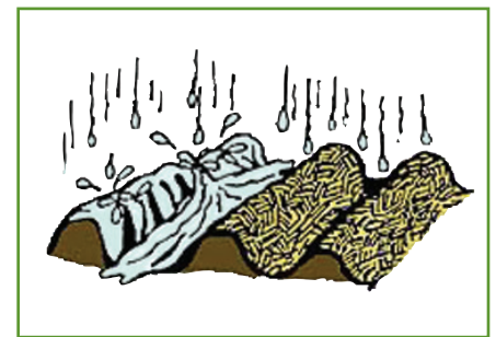
Figure 1. Mulch resists splashing raindrops and erosion.
